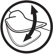
To turn the seat, depress and hold down the seat swivel lever at the side of the seat pad. This will then allow the seat to be rotated to face the staircase landing. The seat will lock in position at 45° and 80°.
