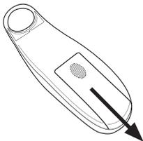
Slide the battery cover off the reverse of the remote control.
