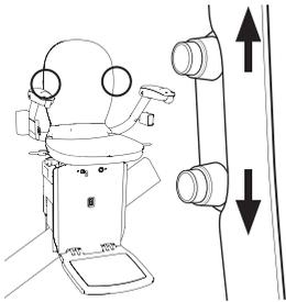
If a Powered Footrest is fitted, at the top or bottom of the stairs, after the stairlift comes to a stop, undo the seat belt and leave the stairlift. Using the buttons located along both sides of the seat, lower or raise the footrest as required. Alternatively, the Powered Footrest can be raised by pressing both buttons of the remote handset at the same time.
